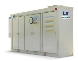
The Power Series all-in-one system is built from paralleled AC string inverters installed inside an air-cooled section of the container, together with an isolated HVAC-cooled DC battery compartment. DC battery strings are aggregated in small groups to keep the DC bus voltage at lower, safer levels for the end customer. The system can operate from 200 VDC up to 1350 VDC, making it compatible with most current and future energy storage technologies.
